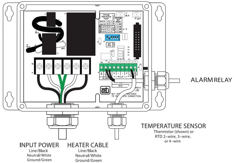
FIGURE 1. The GPT 130 wiring layout.
