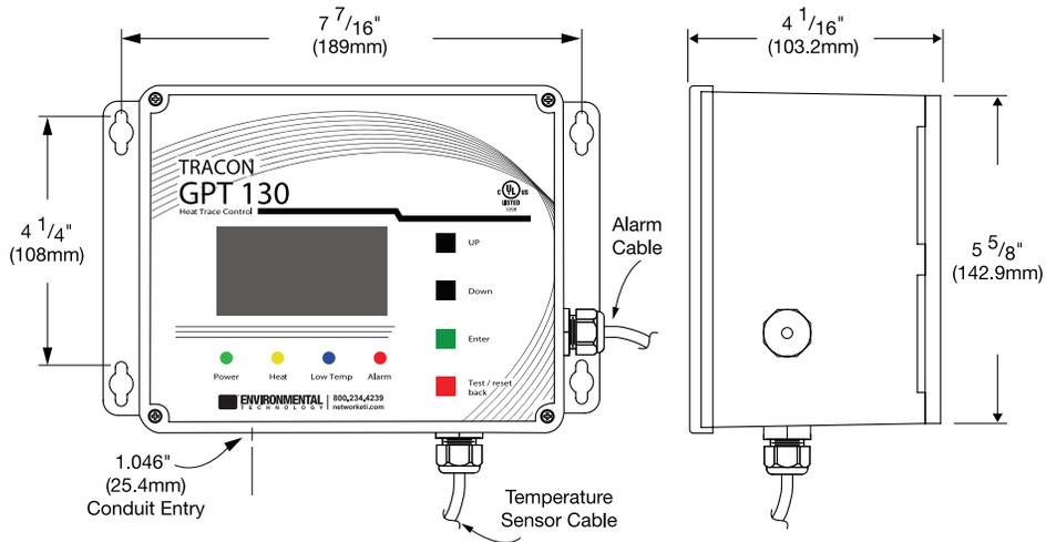
FIGURE 2. Mounting dimensions.
