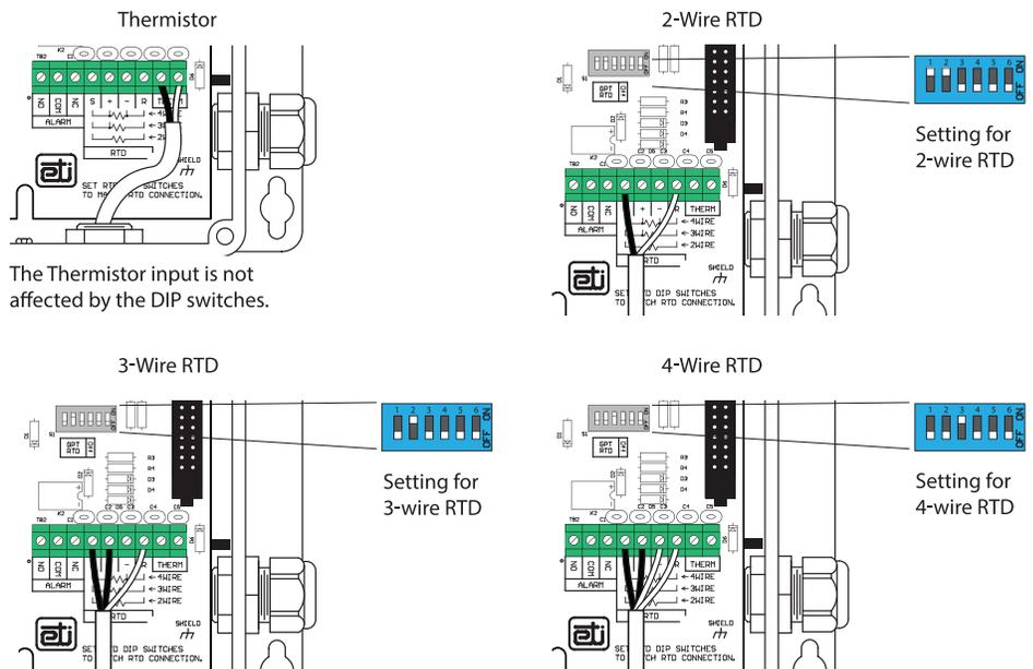
FIGURE 4. Temperature sensor wiring and DIP switch configurations.
