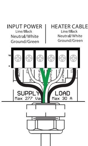
FIGURE 3. Contractor connections.
