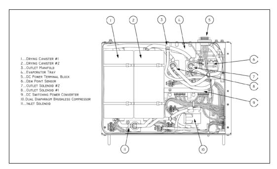
FIGURE 1. ADH NETCOM DC Unit Components.
