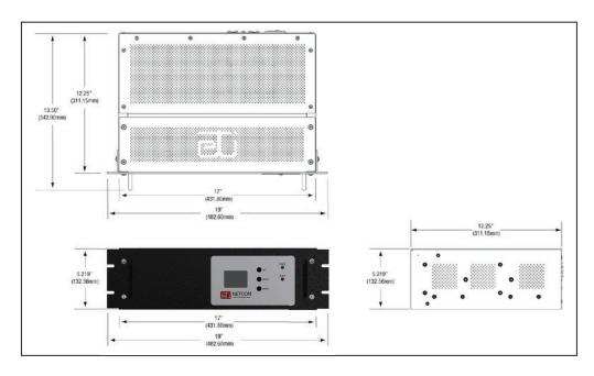
FIGURE 10. ADH NETCOM Rack Mount dimensions.
