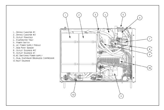
FIGURE 1. ADH NETCOM AC Unit Components.
