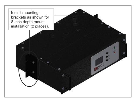
FIGURE 16. Mounting brackets in 8-inch depth position.
