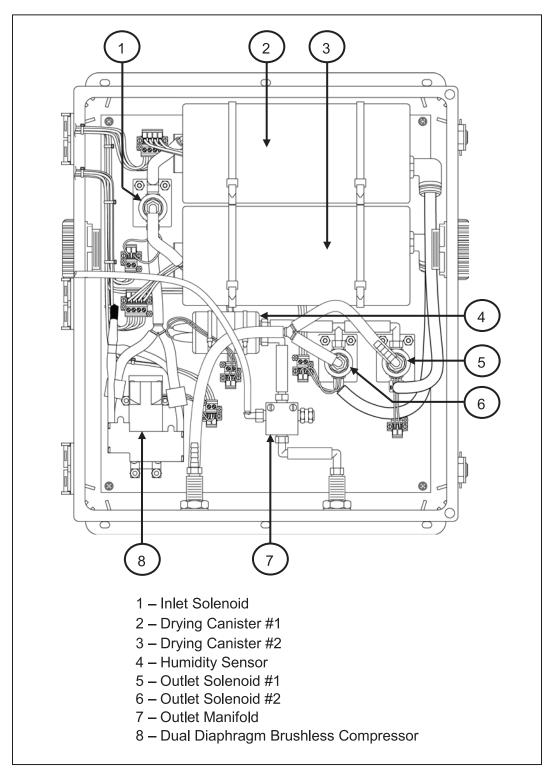
FIGURE 3. ADH NETCOM AC NEMA components.
