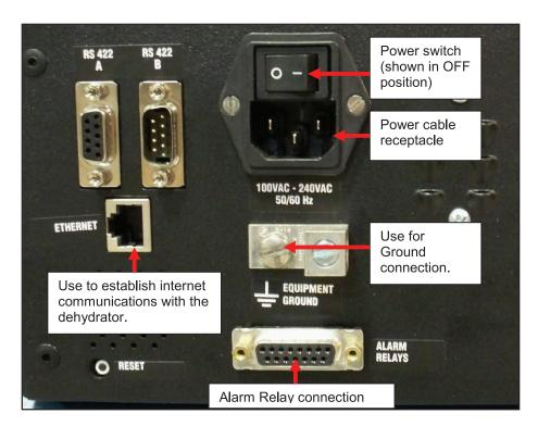
FIGURE 6. ADH NETCOM AC Version Rear Panel Detail.
