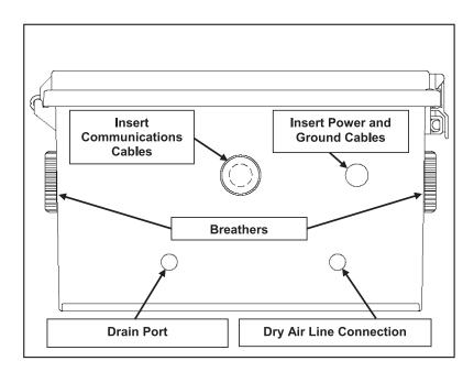
FIGURE 4. Base of NEMA enclosure.
