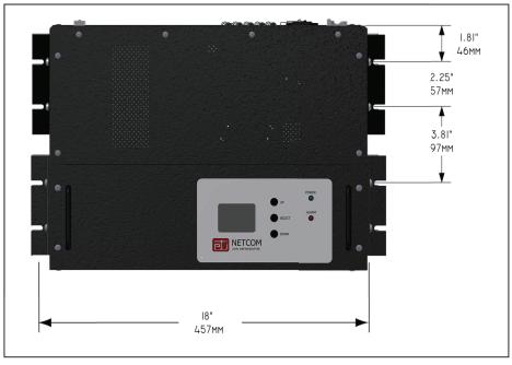
FIGURE 19. Wall mount point dimensions.
