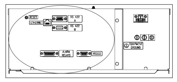
FIGURE 6. ADH NETCOME AC NEMA communications connections.
