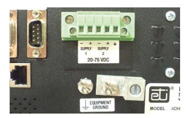
FIGURE 7. ADH NETCOM DC Rear Panel Detail.
