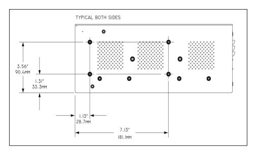
FIGURE 11. ADH NETCOM Rack Mount Hole Dimensions.
