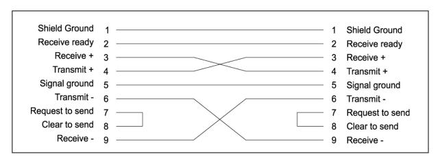
FIGURE 1. Interface cable wiring connection.
