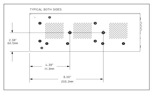
FIGURE 12. ADH NETCOM Slide Rail Mount Hole Dimensions.
