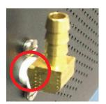
FIGURE 5. Thread Tape on Fitting.
