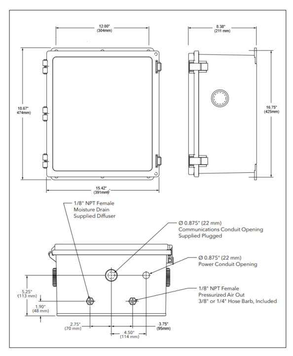
FIGURE 3. The ADH NETCOM AC NEMA enclosure dimensions.
