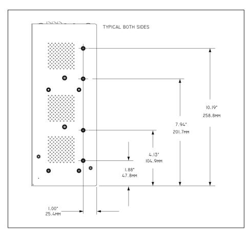
FIGURE 18. Wall mount bracket hole dimensions.
