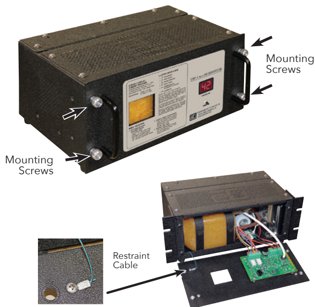
FIGURE 9. Desiccant Bottle Removal - Front Display Panel Mounting screws locations; opened front panel
