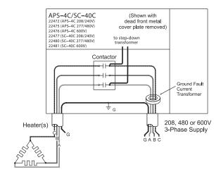
FIGURE 14. APS-4C and SC-40C Three Phase Delta Connection.
