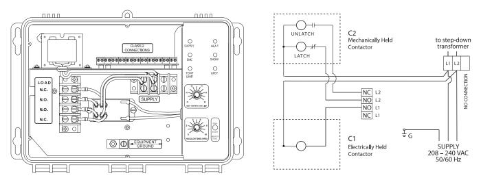
FIGURE 11. 240 VAC APS-3C Operating Mechanically-Held and Electrically-Held Contactors
