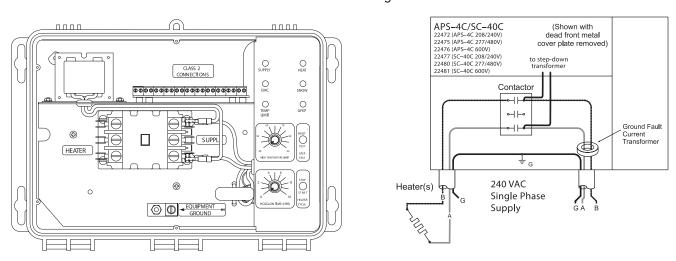
FIGURE 13. APS-4C and SC-40C 240 VAC Single Phase Heater Connection.
