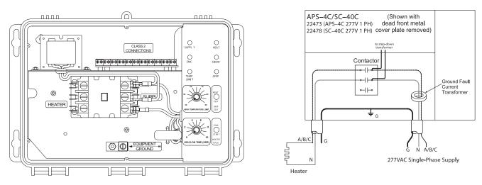
FIGURE 12. APS-4C and SC-40C 277 VAC Single Phase Heater Connection
