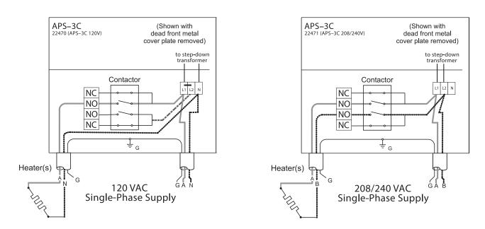
FIGURE 10. APS-3C: 120 VAC and 240 VAC Wiring to Heaters.
