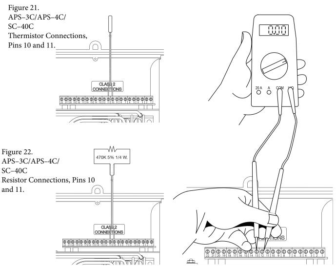
Figure 23. APS-3C/APS-4C/SC-40C Electrician's DVM Connection, Pins 12 and 13.
