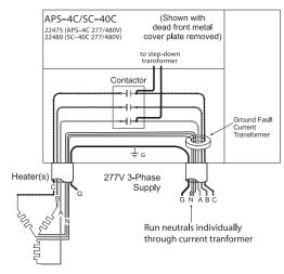
FIGURE 15. APS-4C and SC-40C Three Phase Y Connection(WYE).
