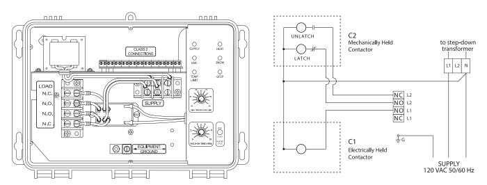
FIGURE 9. APS-3C: Operating Mechanically-Held and Electrically-Held Contactors
