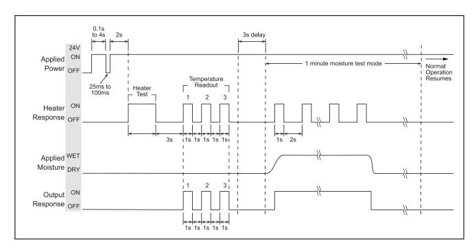
FIGURE 7. Sensor Self-Test Mode.
