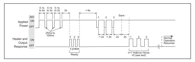
FIGURE 9. Hold-On Time Configuration Mode.
