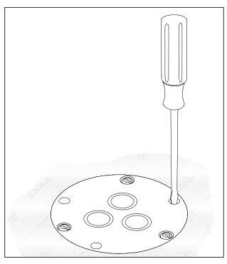
FIGURE 3. Rotate Height Adjustment Screw clockwise to lower or counterclockwise to raise sensor.
