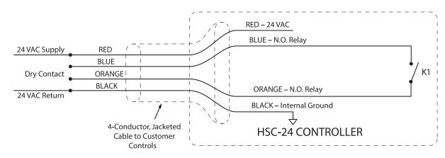
HSC-24 Wiring for Boiler Controllers
