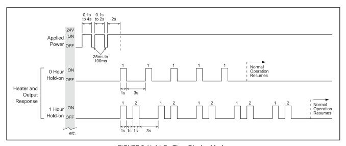
FIGURE 8. Hold-On Time Display Mode.
