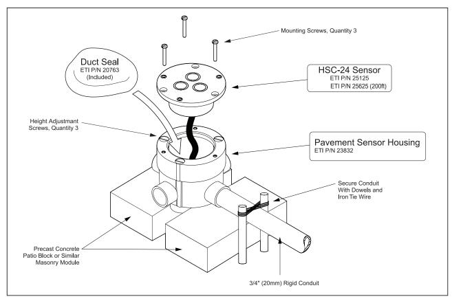
FIGURE 1. HSC-24 Pavement Sensor Installation.
