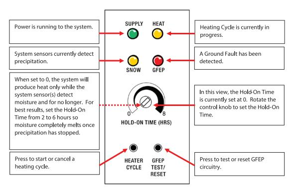
FIGURE 6. The GF PRO Operator Controls and Indicators
