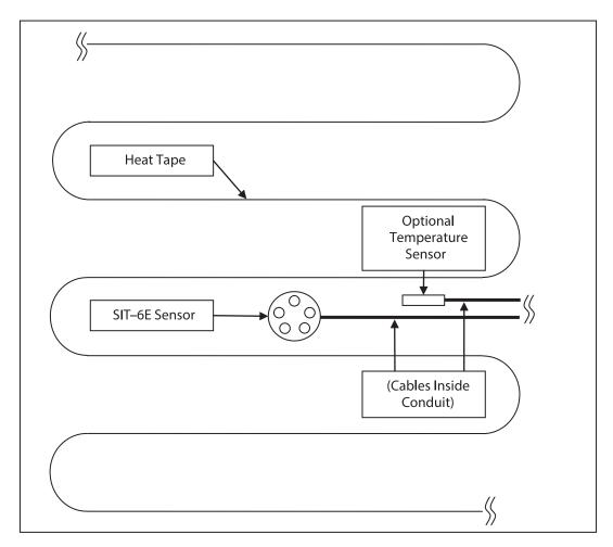
FIGURE 3. Representative SIT-6E Pavement Installation
