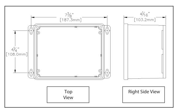
FIGURE 1. GF PRO Mounting Hole Footprint
