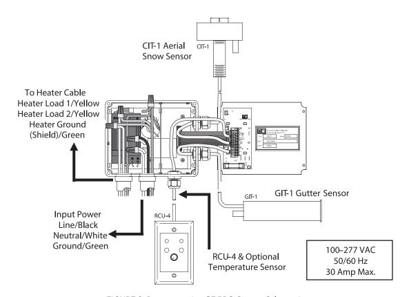
FIGURE 2. Representative GF PRO System Schematic
